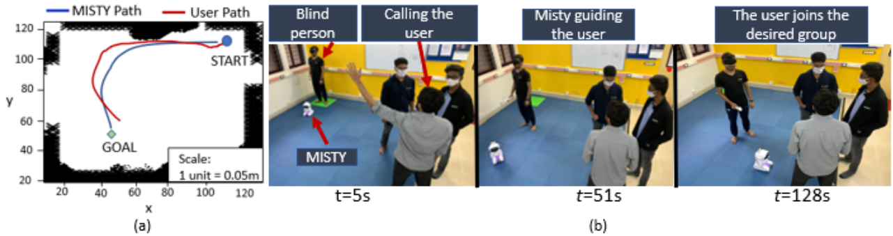
Fig. 11: (a) Path followed by MISTY and the user in an indoor trial depicted on the grid map. (b) Snapshot of the indoor trial. MISTY identifies the person calling the user, estimates the destination and guides the user towards the goal.
